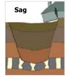
As the roof sags into the mine void, the ground surface will sag correspondingly. As the ground surface sags, it pulls away from the edge of the trough and creates tension cracks around the perimeter. Subsequently, the ground is compressed in the center of the trough and a small ridge can form. The surface tilts where the ground curves into the trough. These movements result in horizontal tension, compression and tilting of the ground surface.
