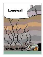
**Longwall** — Longwall mining involves the total removal of coal from a predetermined area. Nothing is left to support the roof and overburden, so subsidence is almost immediate and complete. Unlike traditional room-and-pillar mining, \*once a longwall mine or panel has subsided the vertical movement will cease as the void has been filled.
